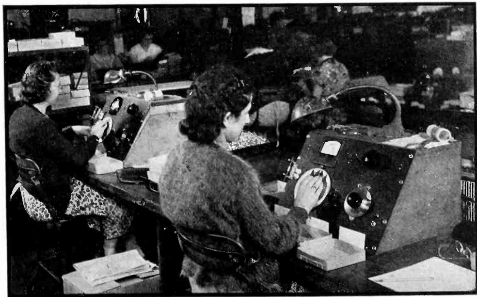
Fig. 9—Apparatus used for checking the capacity and power factor of condensers as the latter are held in a clip at the left of the panel. A dial with limit settings facilitates the measurements
