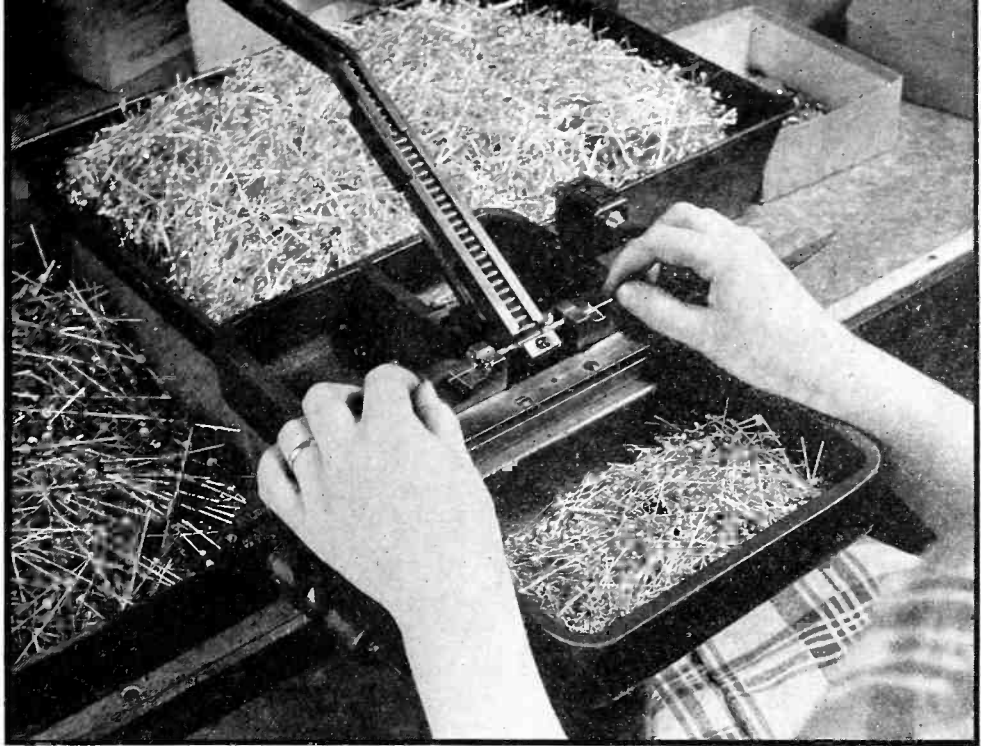
Fig. 7—Fixture used for applying capped wires to the ends of carbons, the latter first having been slipped inside a ceramic case and fed down the chute at the center. Jaws at each side of the chute, brought together by a treadle, force the cups over the ends of the carbon
