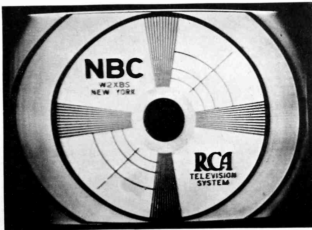
Fig. 9—RCA-NBC test chart, reproduced by the receiver from a one millivolt signal under normal conditions. The actual size of the image was 8 by 6 inches
