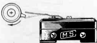
Micro Switch with snap spring actuator operated by cam.
