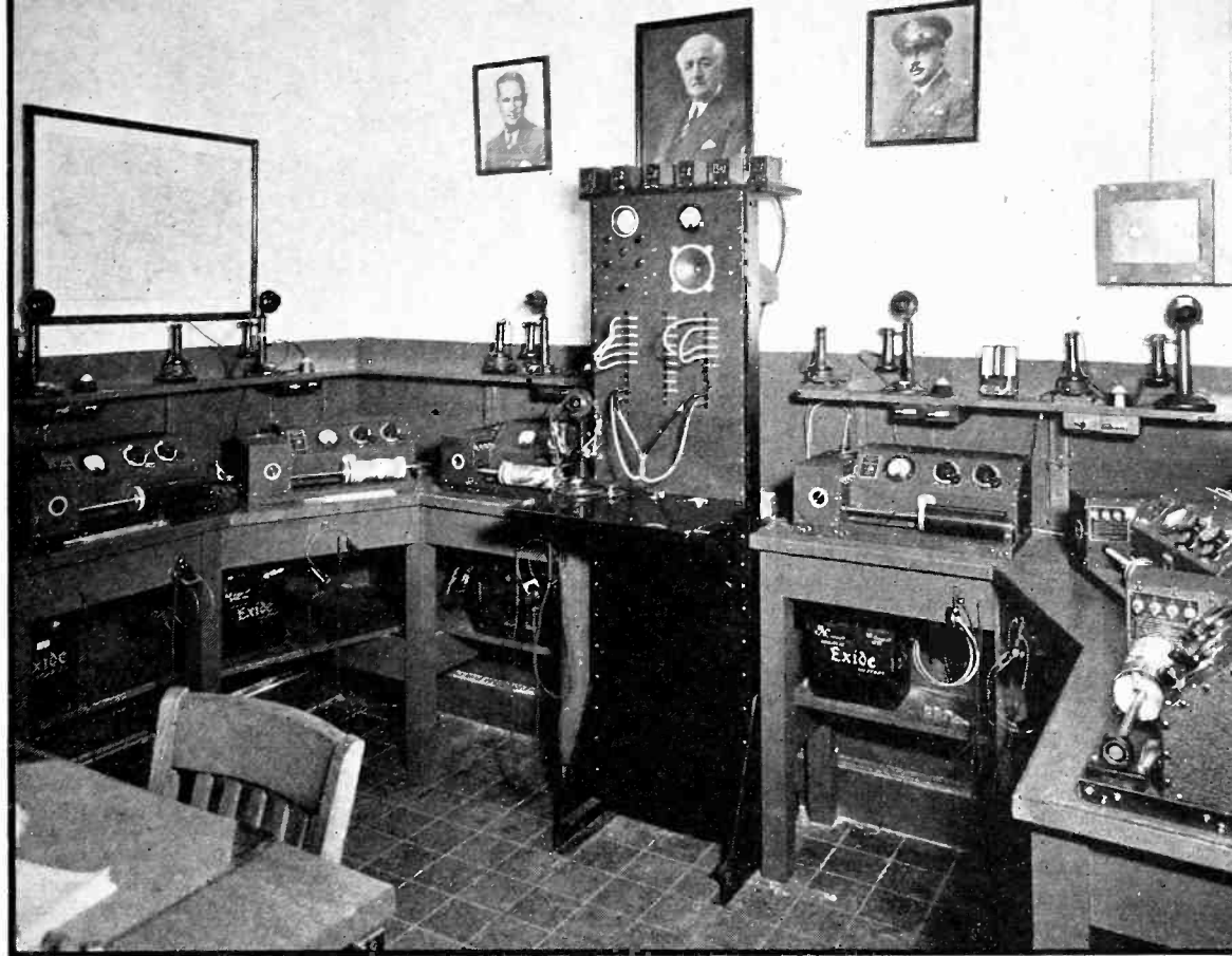
Transmitting room of Wide World Photos. Note the position of the telephone receivers on the coupling coils and the dummy receivers on the telephone hooks. These transmitters are designed to operate from the storage batteries shown under the bench
